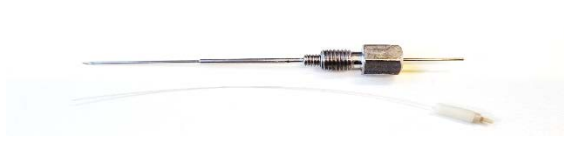
Figure 8: Passivated stainless steel sampling needle without PEEK liner.
