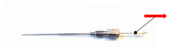
Figure 7: Remove the PEEK liner.
