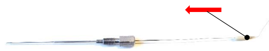
Figure 4: Insert the OFM Fraction Collector Needle Insert into the passivated stainless steel sampling needle (BASi)
