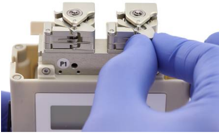
Figure 13: Opening of pump head using the snap mechanism.
