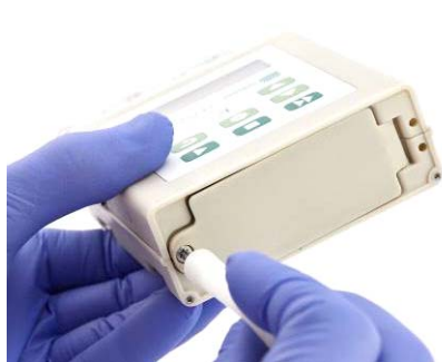
Figure 9: Open the battery compartment with the provided tool.
