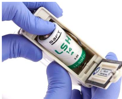
Figure 10: Insert a new battery according to the polarity. The battery removal strip underneath the battery facilitates easier removal.
