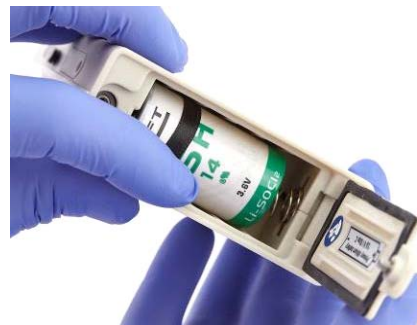
Figure 11: Close the battery compartment cover with the tool by securing the battery compartment screw. Do not jam the battery removal strip.
